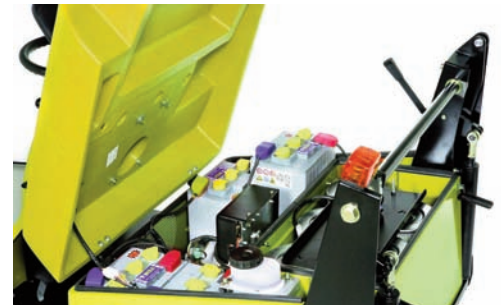
Optional: no. 4 batteries 6v-180ah (5h)
