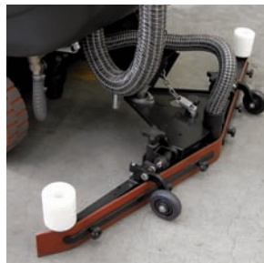
Automatic device for squeegee lifting while reversing.
