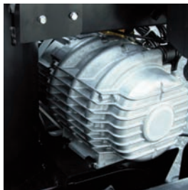
Water cooling* (stainless steel coil) 4 poles electric motor
