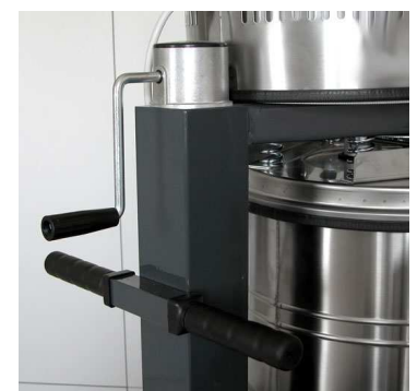
Collector tank lifting system
