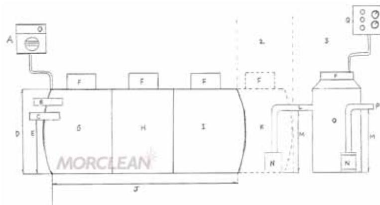
Where the levels and falls are insufficient to outflow to the mains foul drain under gravity, then a Morclean Pumping Chamber can be used.
